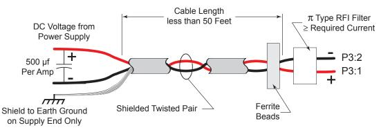
Figure 2.2.3: DC Cabling - Under 50 Feet
